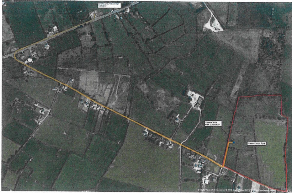
Figure 1: Route of proposed underground cable
